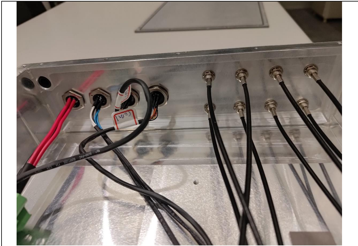
Inside view of enclosure after IPX7 water test (EUT)
